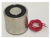
This magnet exerts a holding force of approximately **55 Kgf** perpendicular to any steel plate (see accessories) with which it is in contact, assuming nominal voltage, and coil at working temperature rise of 60°C in an ambient of 20°C.
